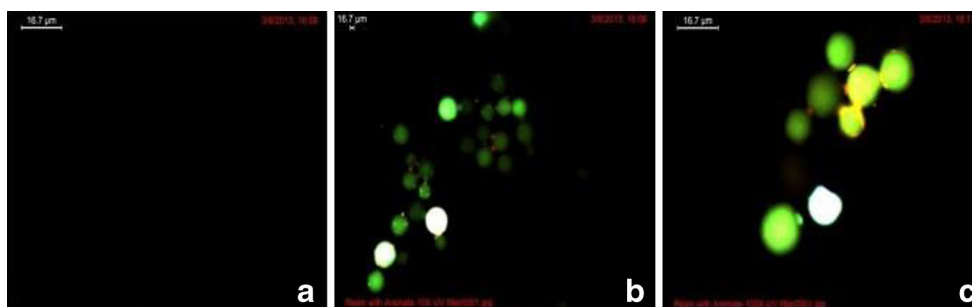
Fig. 22 a Fluorescence microscope images of DFPPIC -Merrifield polymer before sorption of \text{H}_2\text{AsO}_4^- ; b fluorescence microscope images of DFPPIC -Merrifield polymer after sorption of \text{H}_2\text{AsO}_4^- at 10 \times objective lens and c the system b observed under 100 \times objective lens
